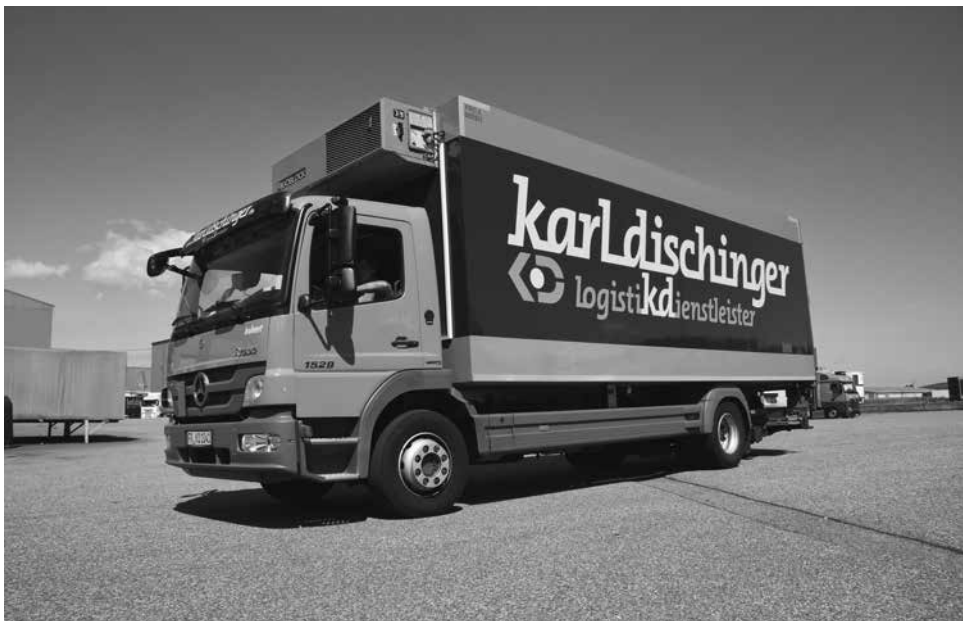
Figure 29.2 A four-wheeled rigid vehicle fitted with a refrigerated body
