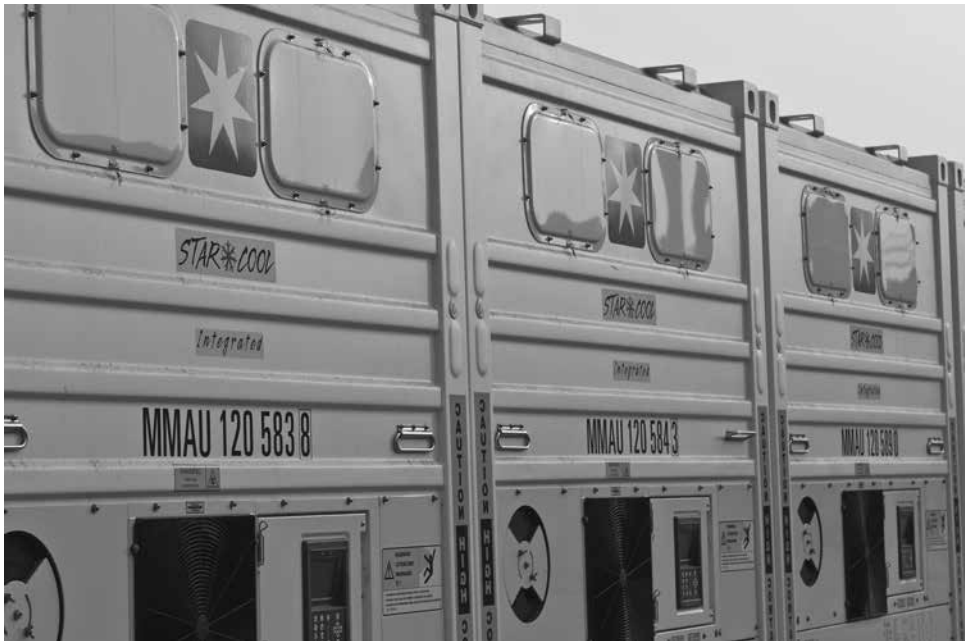
Figure 28.2 Refrigerated containers showing the refrigeration units fitted to the front
