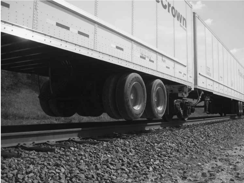
Figure 28.3 RoadRailer® semi-trailers coupled to form railway rolling stock
