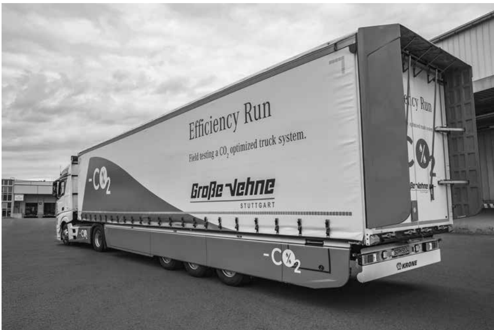
Figure 29.7 An articulated vehicle with a triaxle trailer equipped with aerodynamic mouldings to reduce drag and thus improve fuel economy
