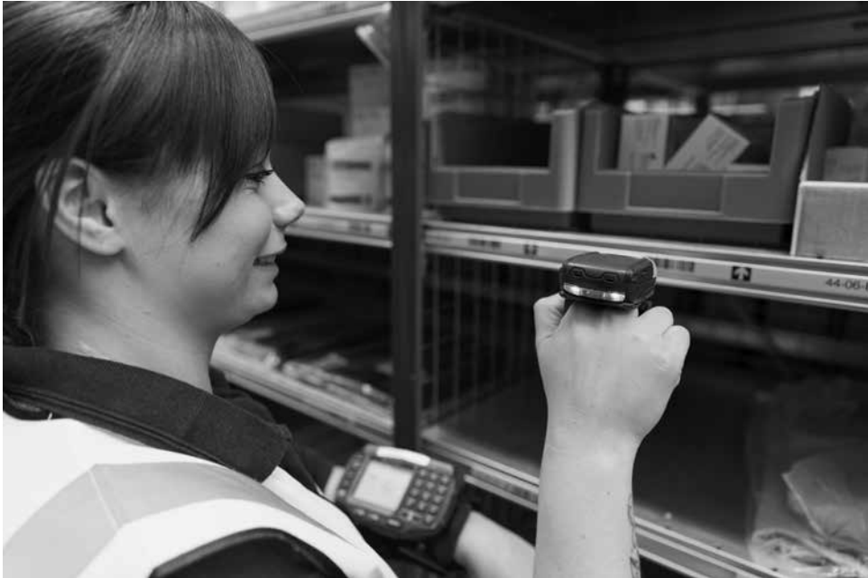
Figure 24.3 Bar code scanning using finger scanner and wrist-mounted radio data terminal
