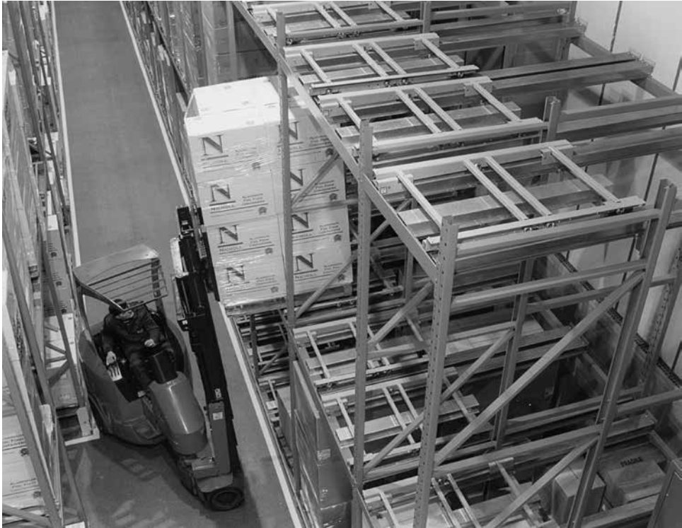
Figure 19.7 Push-back tray racking being served by an articulated fork-lift truck
