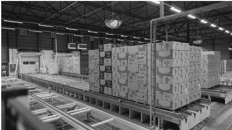
Figure 22.2 Pallets on a conveyor system, ready for automated loading/unloading
