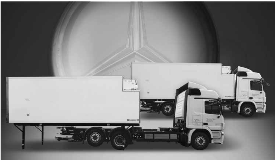
Figure 29.18 Demountable body system
