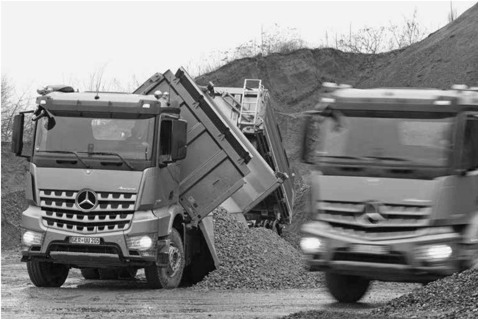
Figure 29.14 A vehicle showing tipping bodies. Note the fact that the vehicle is tipping one container to the side and the other container to the rear of the vehicle
