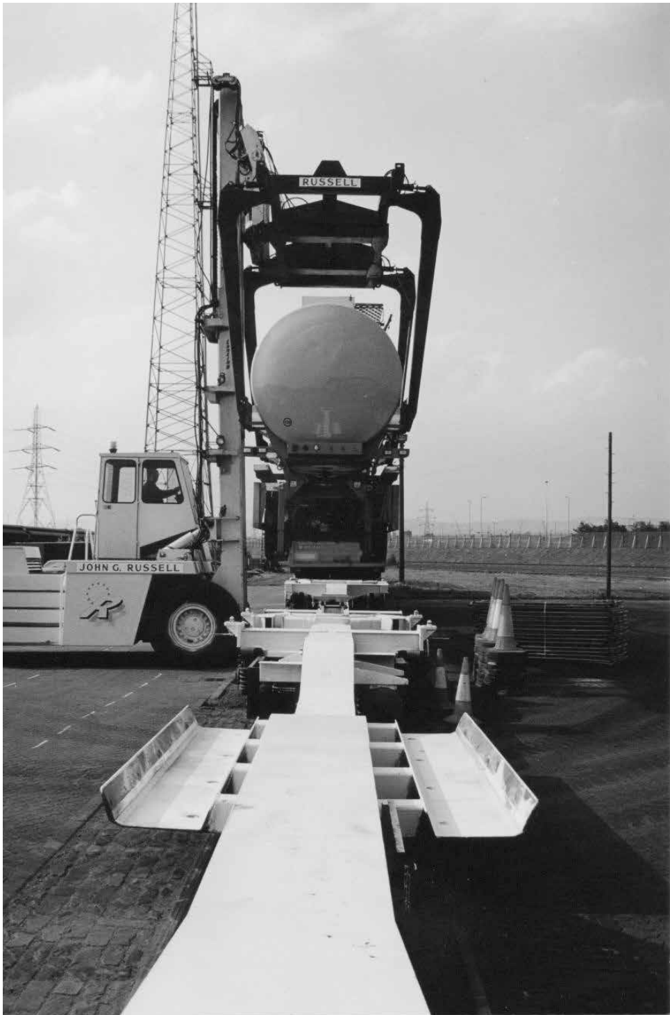
Figure 28.4 Spine wagons being loaded by a reach stacker equipped with a grapple
