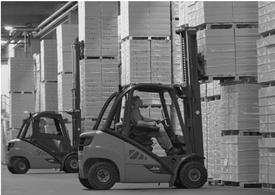
Figure 19.3 Diesel-powered counterbalanced fork-lift trucks block stacking pallets
