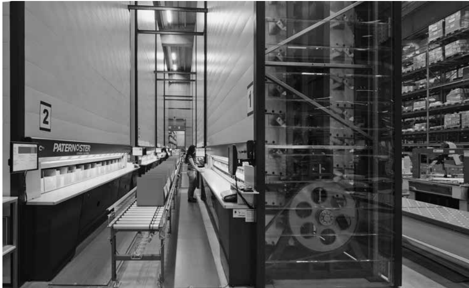
Figure 20.5 Vertical carousel showing the shelf rotation mechanism
