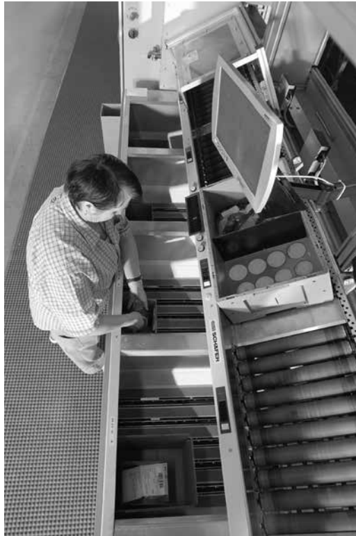
Figure 21.4 Totes-to-picker system with pick by light
