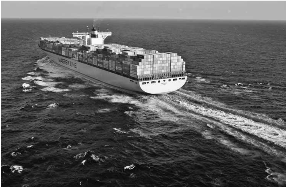
Figure 26.2 The Emma Maersk: one of the largest cellular container vessels in the world, capable of transporting 15,200 TEU
