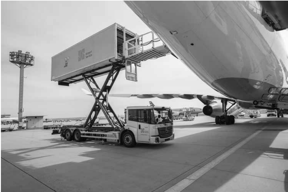
Figure 27.4 An aeroplane being loaded through the side door by a specialist vehicle equipped with a scissor lift
