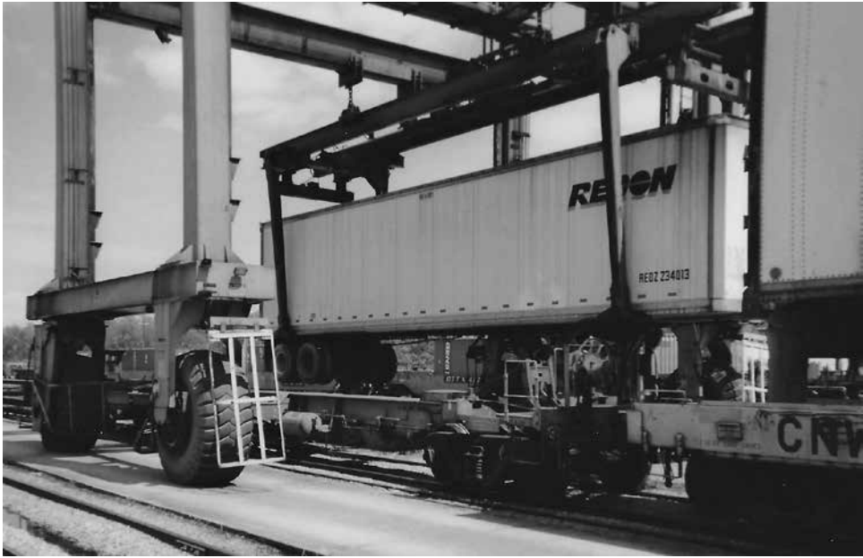
Figure 28.10 A gantry crane with grappler attachment loading road semi-trailers on to rail cars in the USA
