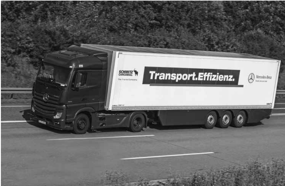
Figure 29.1 An articulated vehicle comprising a tractor and box semi-trailer. Note the skirts on the bottom of the truck to improve fuel consumption
