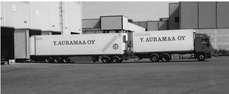
Figure 29.4 A 6x2 rigid vehicle towing a triaxle semi-trailer by means of a tandem axled bogie fitted with a fifth wheel coupling. Both vehicle and trailer are fitted with refrigerated bodies. Oulu, northern Finland
