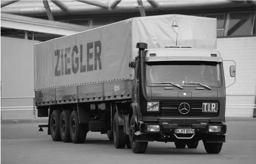
Figure 29.12 An articulated vehicle with a triaxle trailer fitted with a tilt body
