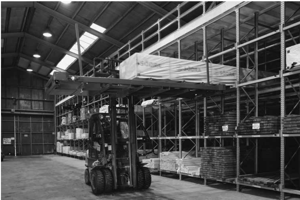
Figure 20.8 Pigeonhole racking being served by a counterbalanced fork-lift truck with specialist attachment
