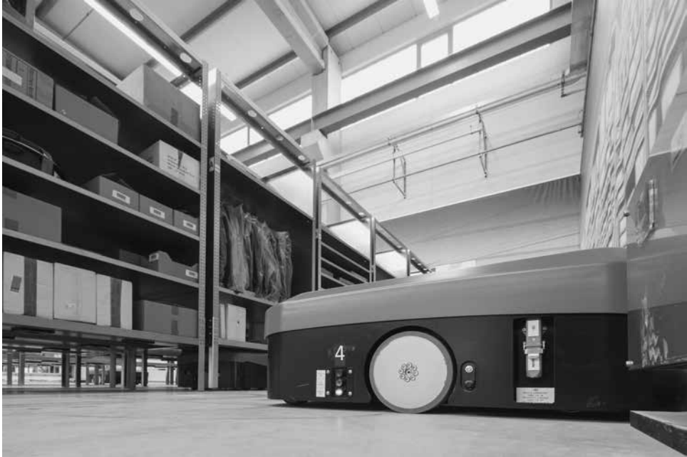
Figure 21.5 Shelf modules-to-picker system showing robotic drive units
