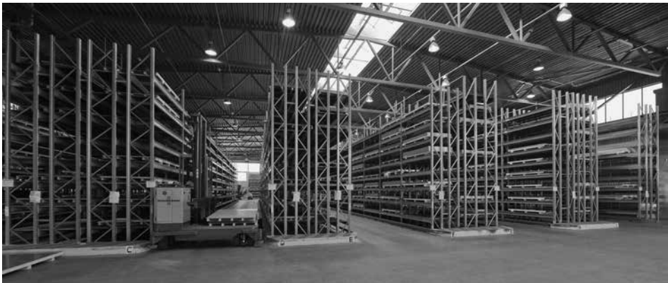
Figure 20.9 Deep adjustable pallet racking for long and wide pallets being served by multi-directional side-loader lift truck
