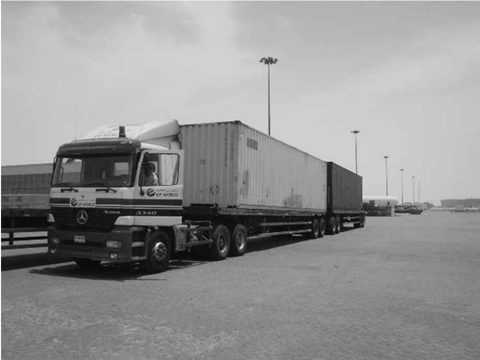
Figure 29.3 A double-bottomed articulated vehicle in Jebel Ali port, UAE
