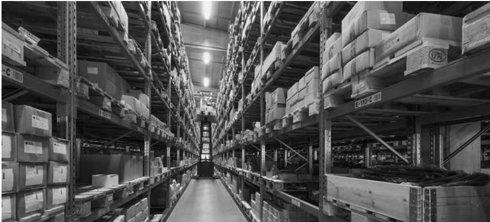
Figure 21.3 Free-path high-level picking truck operating in narrow aisle racking
