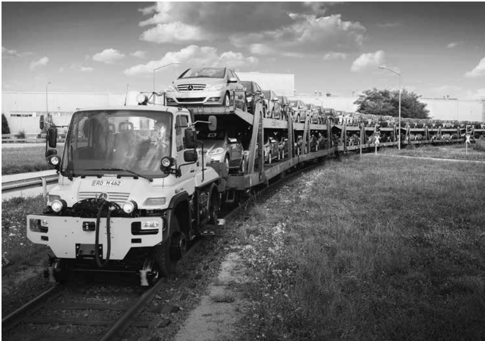
Figure 28.15 Double-decked rail cars loaded with new cars being towed by a converted road vehicle
