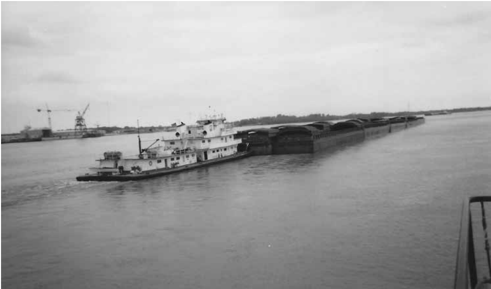
Figure 28.9 River barges being pushed by a powerful tug on the Mississippi River in the USA
