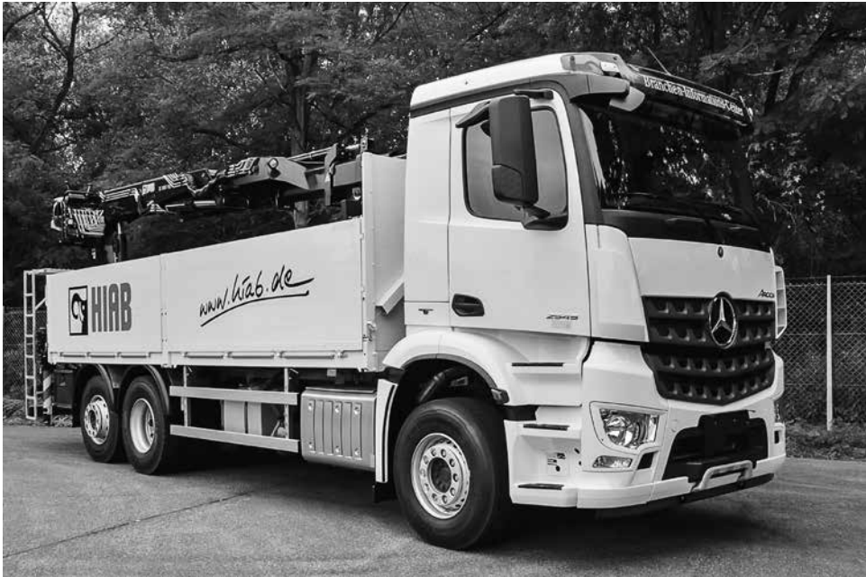
Figure 29.11 A platform or flat-bed 6x2 rigid vehicle with drop sides and HIAB crane to assist loading
