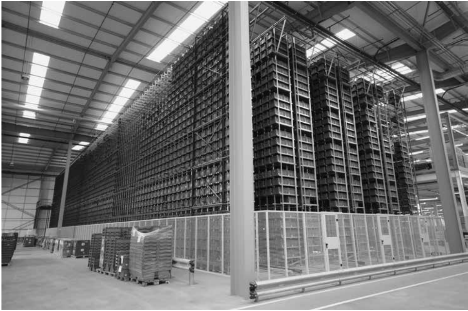
Figure 20.6 Miniload crane tote storage system
