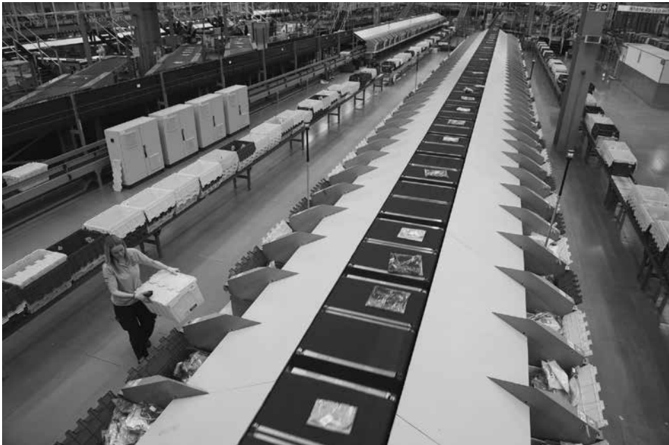
Figure 21.7 Cross-belt sorter showing sortation chutes on both sides
