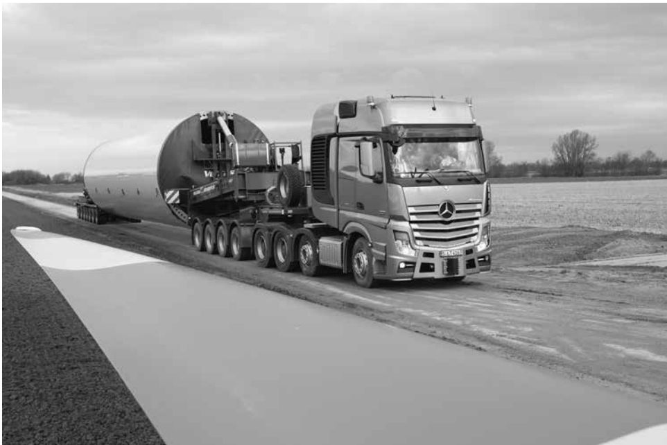
Figure 29.8 A heavy haulage tractor with an indivisible large load
