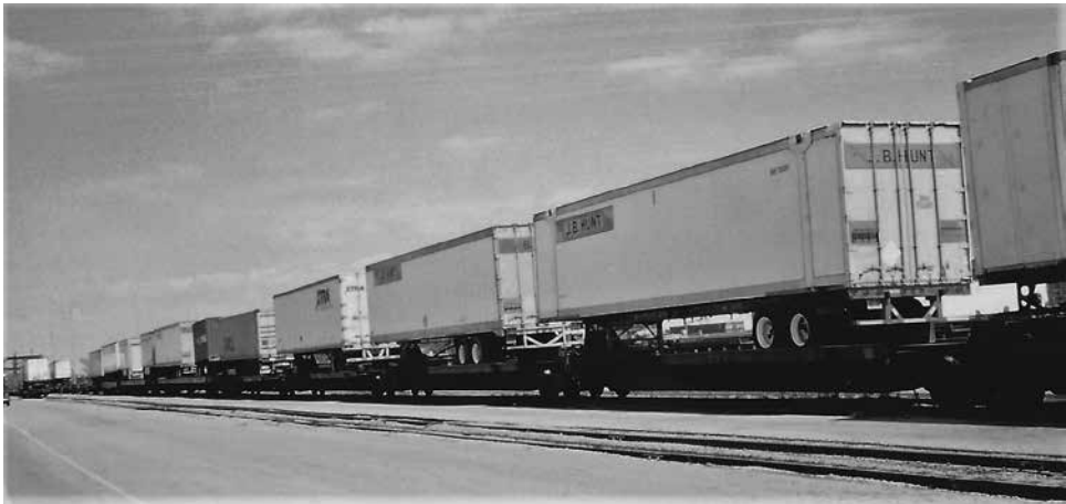
Figure 28.11 Road semi-trailers 'piggy-backed' on rail cars in the USA
