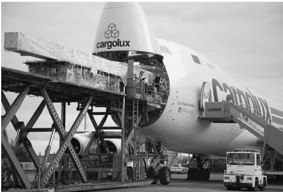
Figure 27.3 An air freighter being loaded through the nose with out-of-gauge cargo
