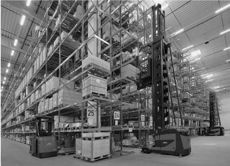
Figure 19.9 Narrow-aisle truck, positioning pallet in a high-level pick-up and deposit (P&D) station
