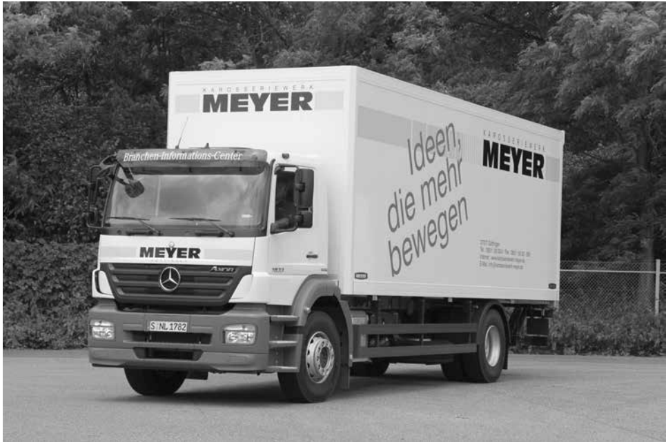
Figure 29.10 A 4x2 rigid vehicle equipped with a box body
