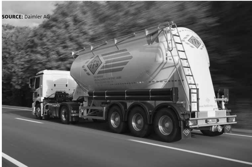
Figure 29.15 A triaxle Feldbinder bottom discharge tanker. The discharge pipe may be seen under the middle of the rear bumper bar
