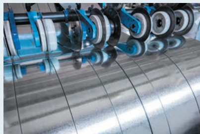
Slitting coils into finished strips.
