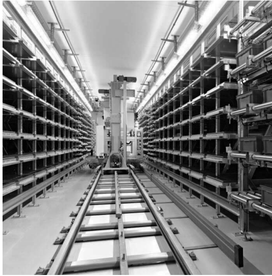
Fig. 4: An example of AS/RS system.
